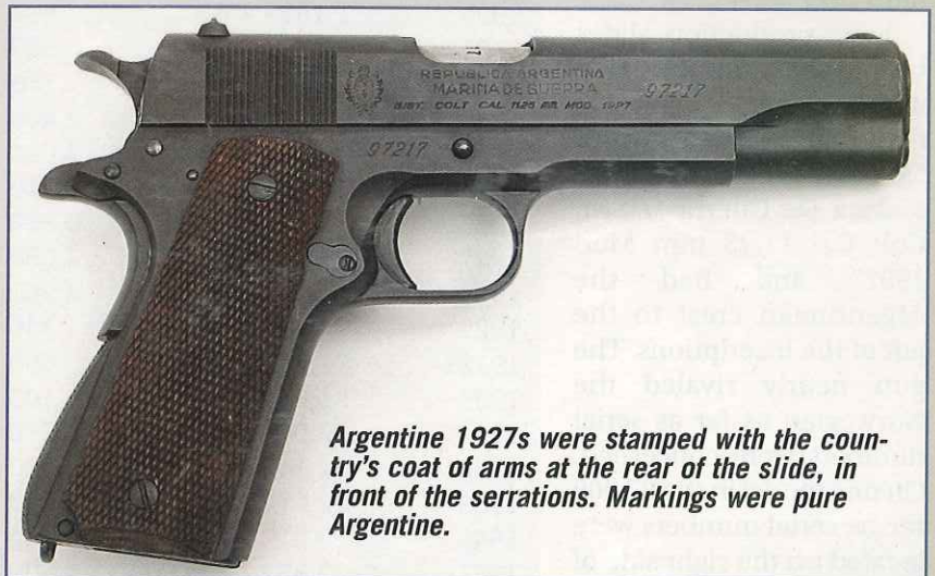
The Argentine Model 1927 was manufactured in Argentina under Colt's license. It was virtually identical to the 1911A1. Unlike the Norwegian 1914, the controls were as seen on the original.
