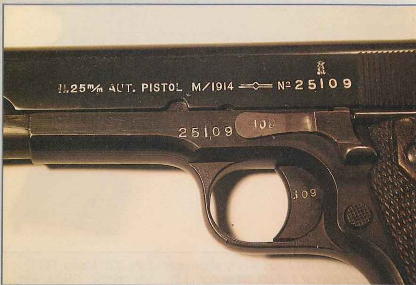
Unlike with the U.S. 1911, all major parts on the Norwegian M/1914, such as this safety and trigger, were serial numbered.
