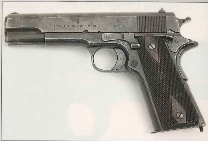
The Norwegian M/1914 was a very close copy of the U.S. Model 1911, with the exception of a slight difference in the slide release. Caliber was 11.25mm (.45 ACP).
